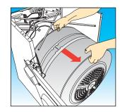
Replacing and/or removing the drum paddle with probe (A320) and/or the drum paddle Step 20 without probe (A310) from the drum assembly (A300):
