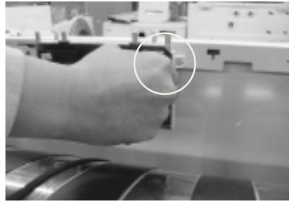
3. Separate frame upper after removing harness at the back.
