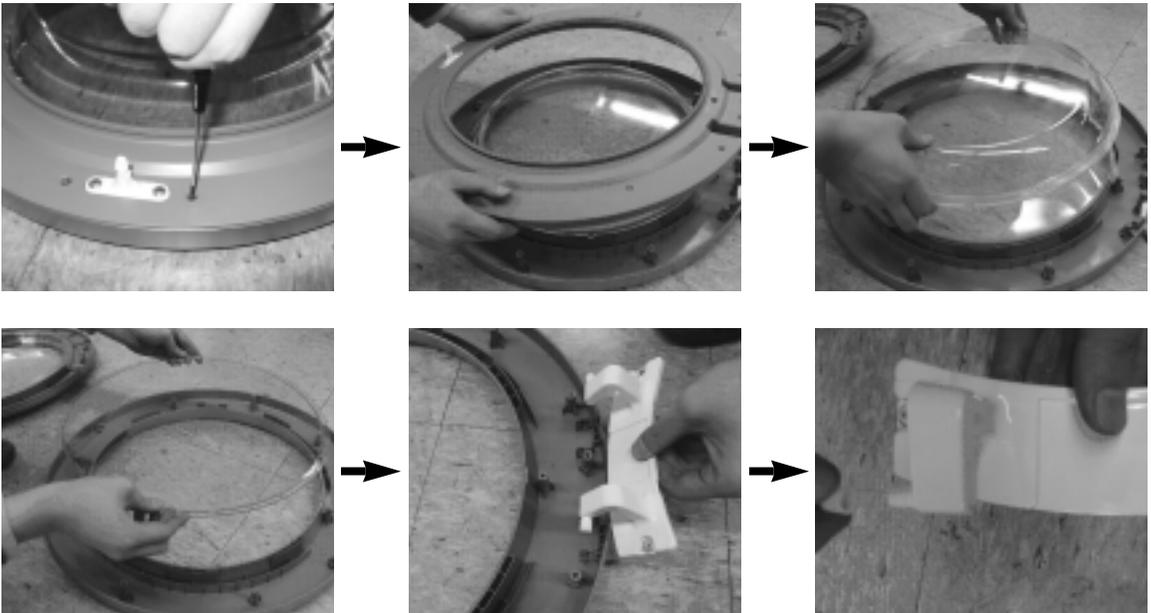
3. Door lock ass'y: Separate door lock ass'y after removing 2 screws.
