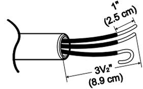
Then, put the hooked shape end of the wire under the screw of the terminal block (hooked end facing rightward) and pinch the hook together and tighten the screw securely.
