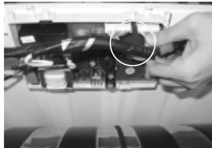
3. Separate humidity sensor connector.
