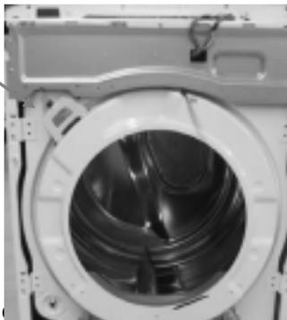
Loosen the screws from the inside of the drum.
