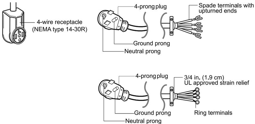
1. Connect neutral wire (white) of power cord to center terminal block screw.
