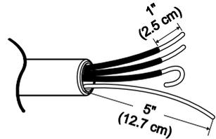
Then, put the hooked shape end of the wire under the screw of the terminal block (hooked end facing to the right) and pinch the hook together and screw tightly.
