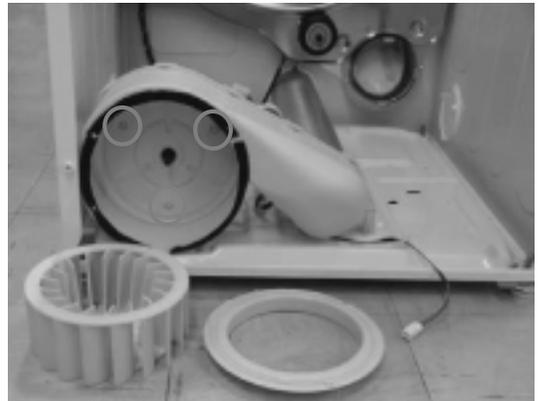
⑧ Remove the 4 screws and the motor ass'y.
