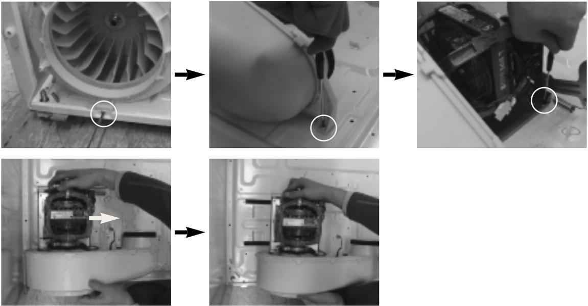
2. Separation of cover fan: Remove 2 screws.
