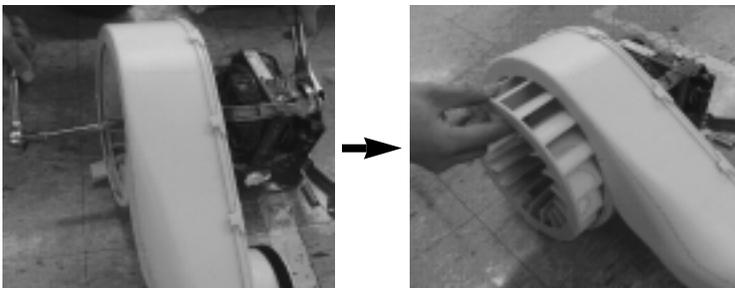
**4. Dismantling of case fan: Remove 3 screws.**
