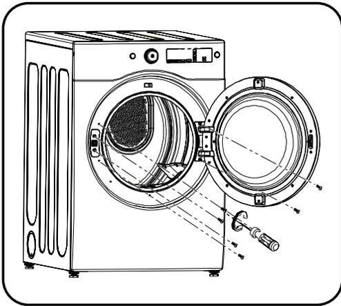
2. Then remove the door out of the front cabinet as indicated by the arrows.
