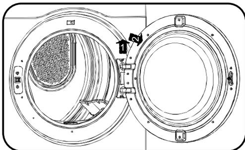
3. Unscrew the four screws on the door lock on the left side of the front cabinet and move to the right side.
