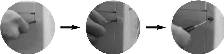
2. Separate panel front. (CAUTION : Internal hook damage attention)
