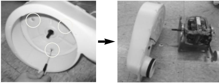
**5. Dismantling of bracket motor: Remove 2 clamp motors each.**
