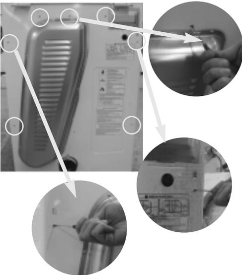
3. Remove support drum rear ass'y in the direction of →
