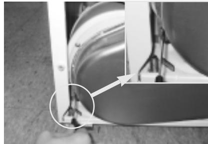
3. Remove duct outlet in the direction of →
