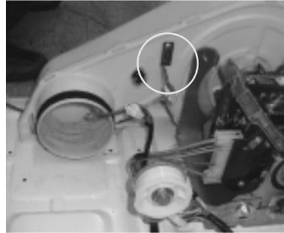
2. Separation of fan thermostat: Separate connector. → Remove 2 screws.
