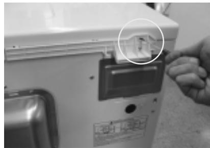
3. Separate top plate by pushing it at the front part in the direction of arrow.
