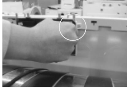
3. Separate and remove the PCB.
