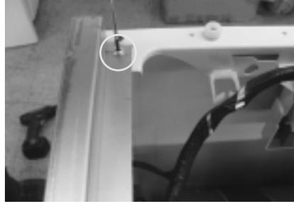
3. Separate upper frame after removing harness at the back.
