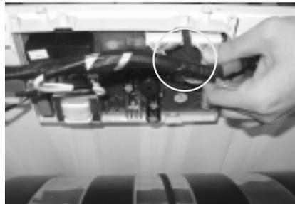
3. Separate humidity sensor connector.
