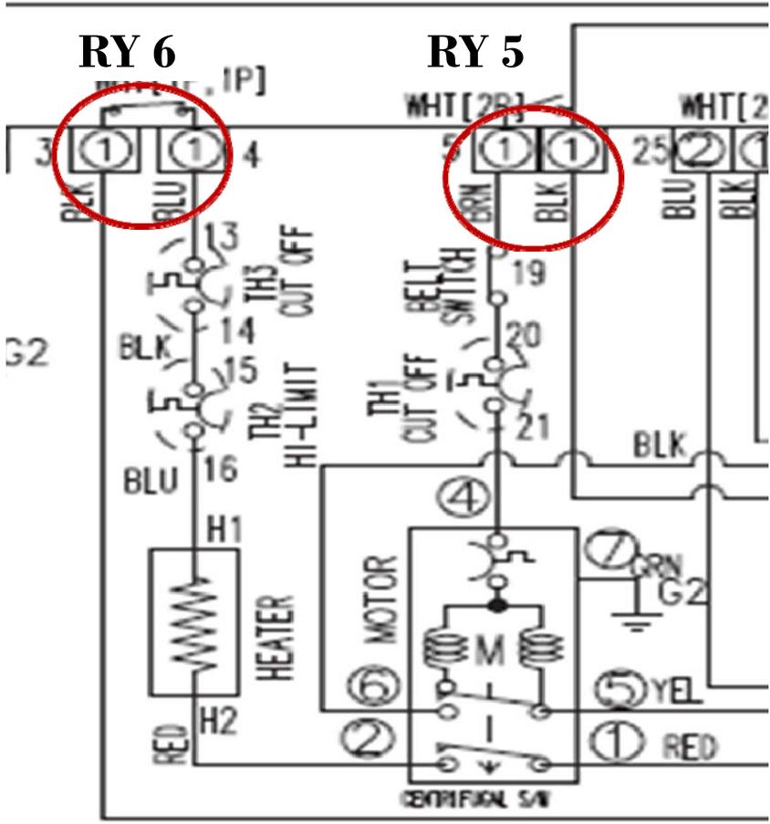
**Testing Main PCB power output to Heating & Motor circuit.**
