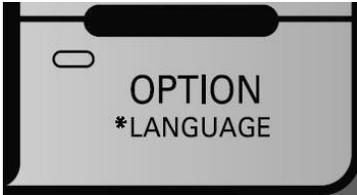
Pressing and releasing the OPTION button opens the OPTION MENU, showing the options that can be added to regular wash cycles.
