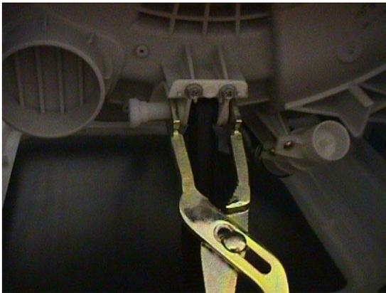
The flat end of the tool goes on the small end and the split end allows the head end to pass through while the pin is pushed out. Sometimes you can use a socket to hold the pin down while you press the pin out.
