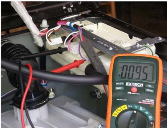
In this picture we see the meter displaying less than 1.5 V<sub>DC</sub>. In this example, the water in the housing is touching the high water sensor probe and the ground probe. When this occurs, conductivity through the water is measured as a voltage drop and the control board knows the water housing is full of water.
