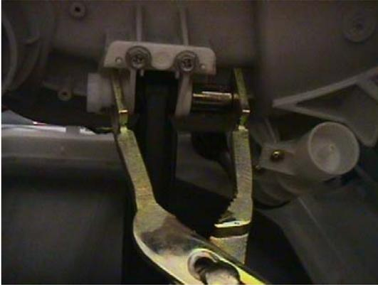
Disconnect the dampers from the tub and the base.
