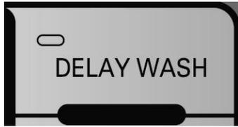
After the cycle is set, press the DELAY WASH button from 1 to 19 times and it will delay the start of the cycle between 1 and 19 hours.
