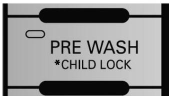
Press PRE WASH to add a pre wash cycle to almost any wash cycle. Add one half as much detergent you would use for a regular wash cycle into the prewash compartment of the dispenser.
