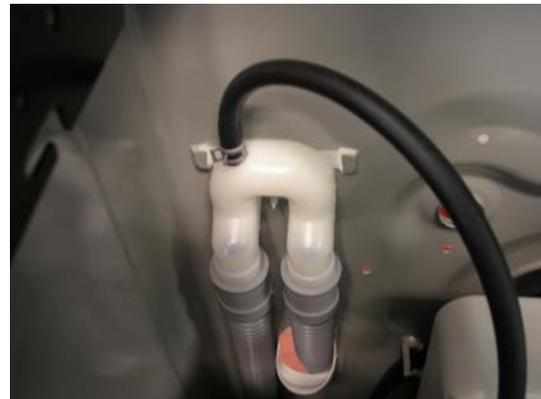
The drain pipe should be firmly attached to the standpipe or the laundry tub or sink where it drains. The pump has sufficient power to cause the pipe to move around when the water is expelled. The pump can lift the drain water a maximum of 96 inches (2.4 m), but there is no minimum height requirement. The vacuum breaker in the drain line will prevent drainage by gravity or siphoning. The hose can lay flat into a floor drain as long as the end of it is not submerged.
