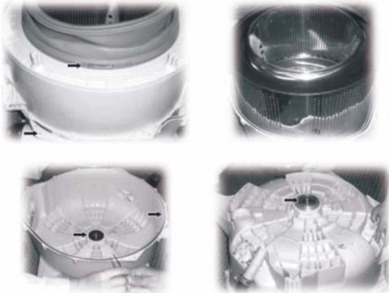
Removing the tub/drum assembly is major surgery. It is much lighter if you remove the weights and the motor. Generally speaking, you'll have to remove all that anyway.
