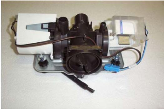
Both the drain pump (left) and the circulation pump (right) are mounted on the filter housing. The entire pump assembly is then mounted on a suspension plate base attached to the washer base by three antivibration bushings and 10 mm bolts. Use a socket and a short extension to remove the pump assembly.
