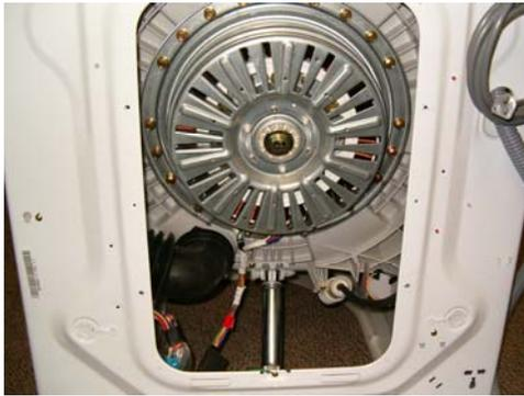
The motor is a direct-drive, brushless, DC motor. It is attached to the drum via a splined shaft, eliminating belts, pulleys, transmissions, and the inherent problems associated with them. The rotor is attached to the shaft by one large bolt.
