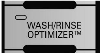
Press WASH / RINSE OPTIMIZER® to make the machine set the optimum water level, wash time, rinse time, and detergent level. The machine will adjust the washing and rinsing times according to the amount of detergent used and the hardness of the water.
