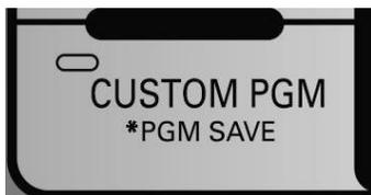
This button activates a custom program created by choosing a cycle and overriding some of the settings using the option buttons. When the program is determined, press and hold CUSTOM PGM for three seconds until it beeps twice. Thereafter, this button will run that custom program. You can overwrite any custom program by simply inserting another custom program.
