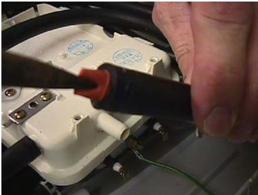
Be particularly careful when removing and replacing the water input hose to the steam generator. There is a check valve that fits into the input port. The valve sometimes comes off and is stuck in the hose. This could cause the water not to flow, which would cause the steam generator to malfunction.
