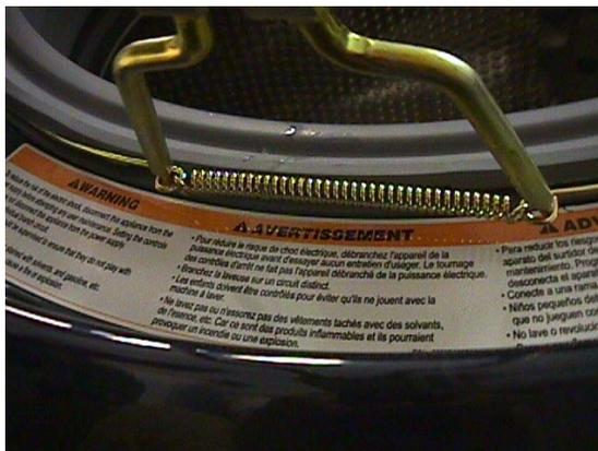
Remove the door gasket using special tool **383EER4001A** to remove the outer spring clamp.
