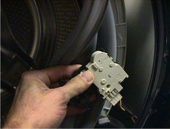
After removing the door gasket, you can reach inside the cabinet and unplug the electrical connector to the door switch.
