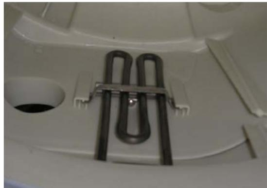
When replacing the heater, be sure the element slides into the retaining clip on the bottom of the tub.
