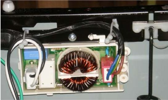
To service the noise filter, remove the control panel cover.
