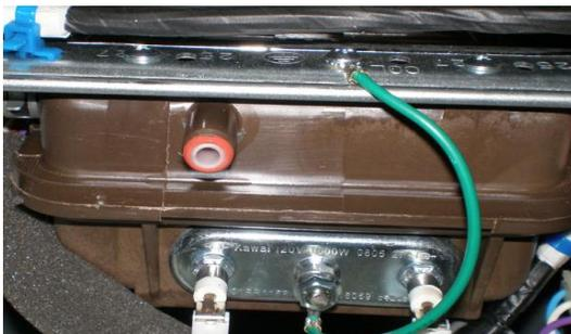
Newer models have a retainer built into the check valve to eliminate this issue.
