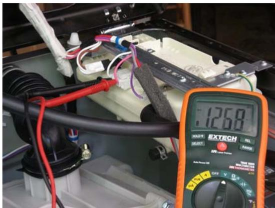
The sensors operate in a 5 V<sub>DC</sub> environment. When water is present and conductivity exists from the white GROUND lead and the pink low water sense lead, less than 1.5 V<sub>DC</sub> will be measured.
