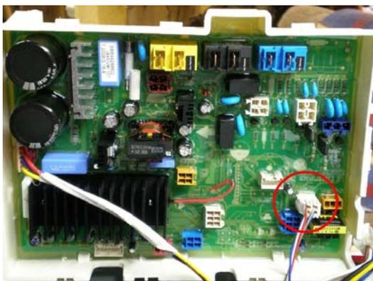
Before going to this trouble, check the connector on the main board. It is the white connector (circled in red.) Pull the connector off and verify the board is receiving a signal from the hall sensor. (See pages 79 ~ 83 for more information.)
