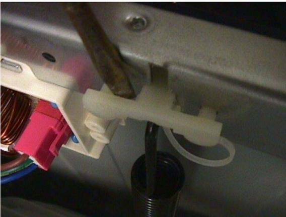
Separate the three dampers. (See page 51.) You can remove just one end now and the other end after the drum is out of the machine.
