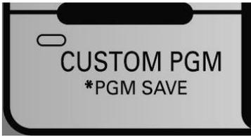
When the user inputs a custom program, press and hold CUSTOM PGM for three seconds until it beeps twice. Thereafter, this button will run that custom program.
