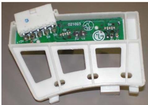
The hall effect sensor is easily removed and replaced. You'll have to remove the rotor and stator to access the sensor. When replacing the rotor, the drum may move forward enough to make replacing the bolt difficult. Carry a longer bolt in your toolbox to use to install the rotor, then remove and replace it with the factory bolt after the shaft has been pulled back and the rotor is pushed in place.
