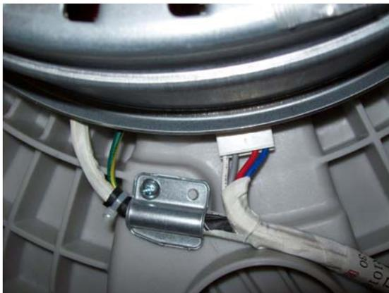
When re-installing the stator, the clamps and the ground screw must be installed and the connectors pressed into place before the rotor is bolted onto the shaft.
