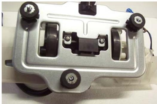
Bottom view of the pump and filter assembly, showing the antivibration bushings and bolts and the two screws that hold the pump assembly to the base.
