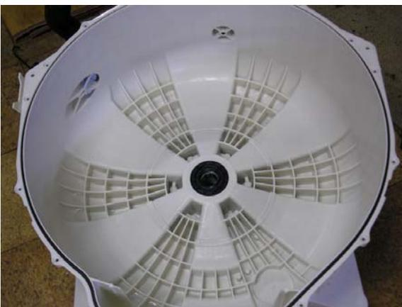
Unbolt the bolts around the circumference of the seam. (top photo) Separate the halves. Be careful to avoid damaging the gasket. Do not pry on the surfaces between the halves.
