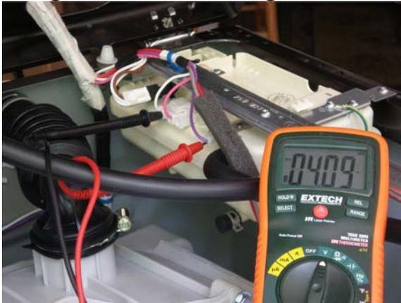
The photo to the left shows the high water sensor (VIOLET) wire. As the caption shows the meter is reading a voltage of 4.09 V<sub>DC</sub>. Water in the housing is not touching the high water probe. When this occurs, the control board would activate the cold inlet valve for the steam generator before energizing the heater, IF steam was selected and the control board wanted steam.
