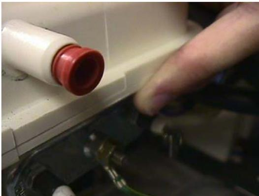
Pull the check valve out of the hose gently and replace it into the water input port. Then slide the hose onto the port and install the clamp.
