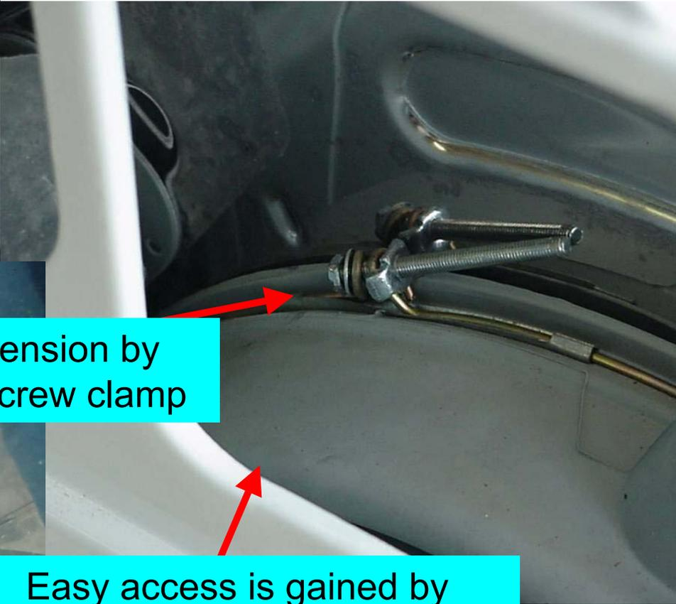
Release tension by removing screw clamp
