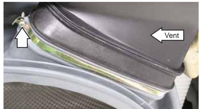
8. Loosen the 7-mm bolt that holds the wire and bolt assembly to the outer tub lip. Remove the wire and bolt assembly from the tub gasket.
