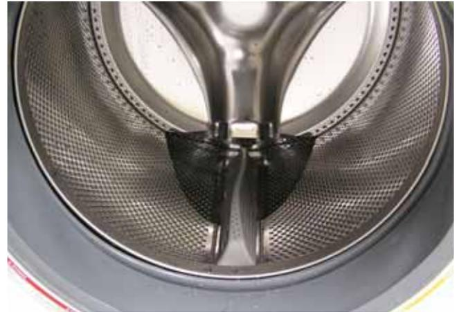
The main water level is approximately 3 inches deep measured behind the baffle and approximately 1¾ inches deep measured at the bottom center of the wash basket.
