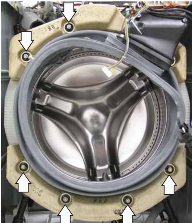
15. Remove the 8 bolts from the slots in the outer tub.
