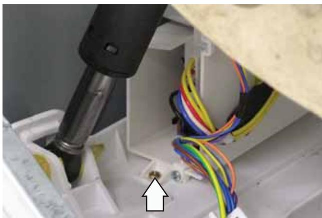
3. Slide the inverter rearward to clear the guides that hold the rear of the inverter to the chassis.
