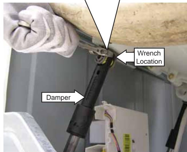
4. Remove the pin that secures each damper to the chassis by pressing the lock tab while pulling the pin out.
