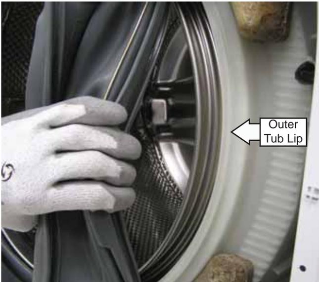
**Note:** When reinstalling the tub gasket on the outer tub, align the indicators on the top and the bottom of the gasket with the arrows located on the top and the bottom of the tub.
