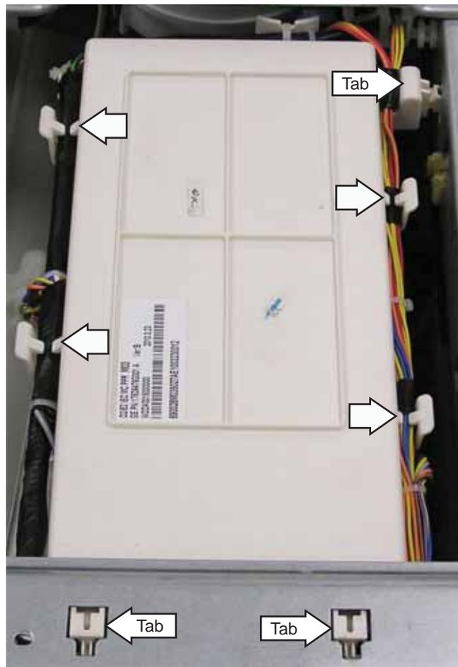
6. Remove the wire tie from the back end of the power board housing.
