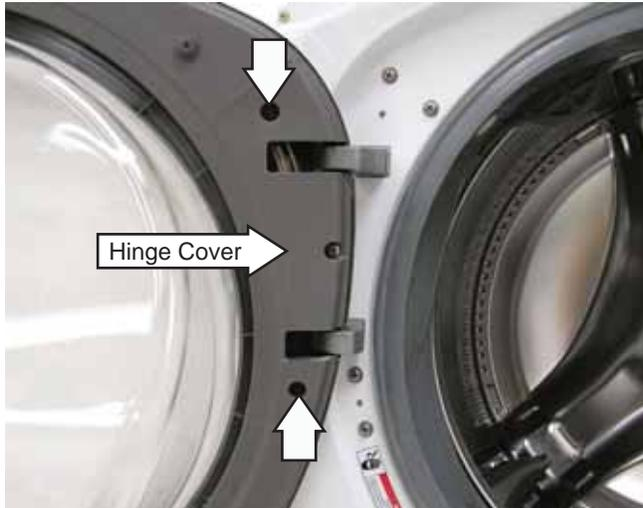
2. Remove the 2 Phillips-head screws that hold the door to the hinge door plate.
