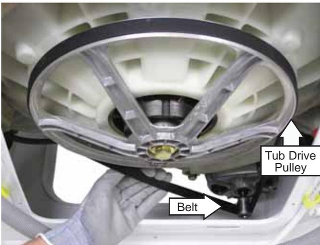
**Note:** The belt is elastic and designed to be removed and installed in this manner.
