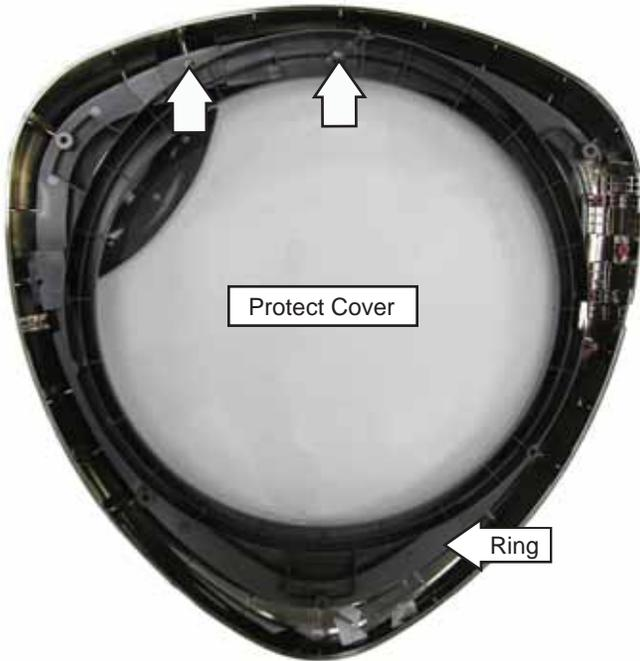
7. Lift and remove the protect cover and ring.
