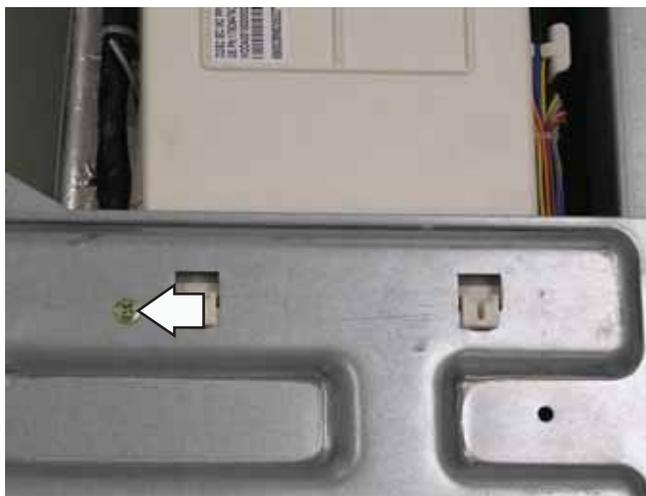
3. Remove the 3 compression tabs from the front brace.
