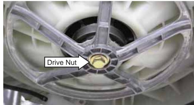
**Caution:** When installing, use a torque wrench to tighten the 18-mm hex nut to 44 ft. lbs of torque.
