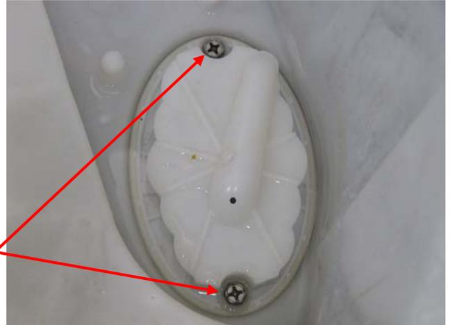
**Note: It is important that the screw bosses are kept free of grit. If the bosses have any grit, this can reduce the travel of the screw, which will lead to a poor fit of the cap, which in turn will cause bypassing (refer to Section 4.9.11). Bypassing can cause water on the floor, especially if the water dribbles from the recirc nozzle on to a spinning bowl.**
