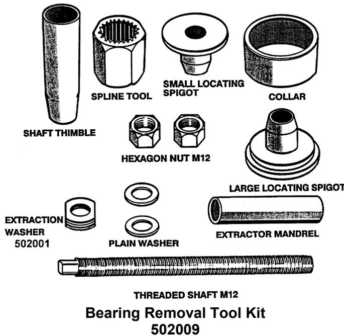
**Note:** *The extractor mandrel was designed for the older shaft with the external thread, however will work with the shaft on this machine with the internal thread.*
