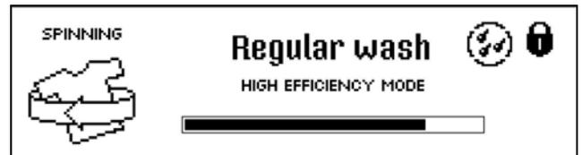
The Lid Lock symbol (padlock) appears in the top right hand corner of the screen on LCD models, and in the centre left next to the power button on the control panel on LED models, letting you know at a glance if you can open the lid or not.
