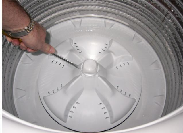
**Note:** *If the low profile agitator does not lift off easily, hold the top balance ring of the inner basket, and then jerk the bowl upwards. This action will push the agitator upwards.*
