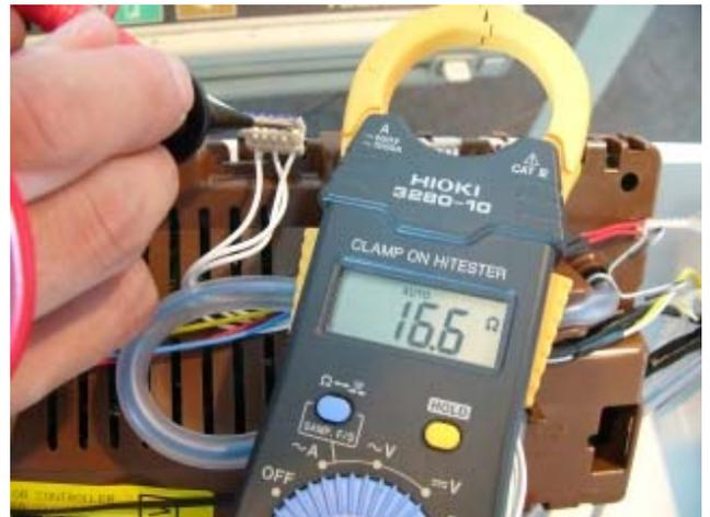
If the meter shows an incorrect reading, we would recommend testing the stator from underneath the machine, as there could be a fault in the wiring harness. To test the stator it will need to be removed from the machine (refer to Section 10.19).
