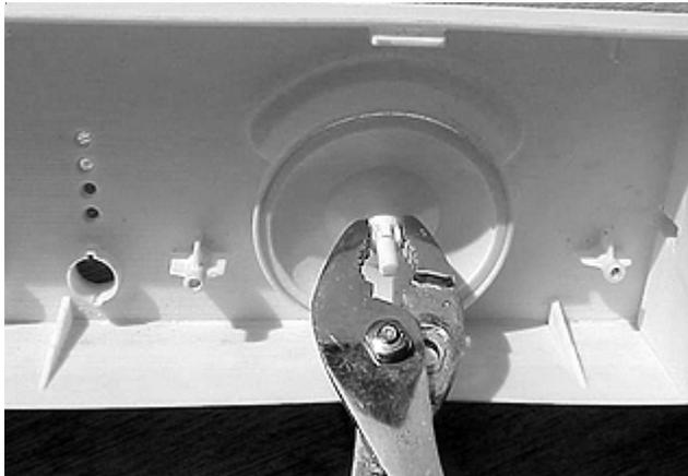
**Note:** Do not use a screwdriver to pry the dial off because it will scratch the dial.
