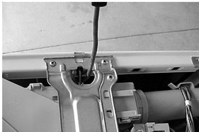
To do this, a strong rod at least 8" long with a hook on one end and a handle on the other is need, such as the one shown here made from a paint roller.
