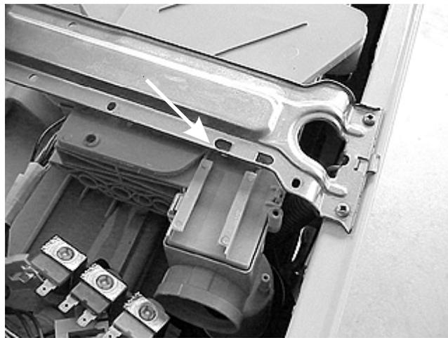
6. Remove the (2) screws holding the housing to the console panel.
