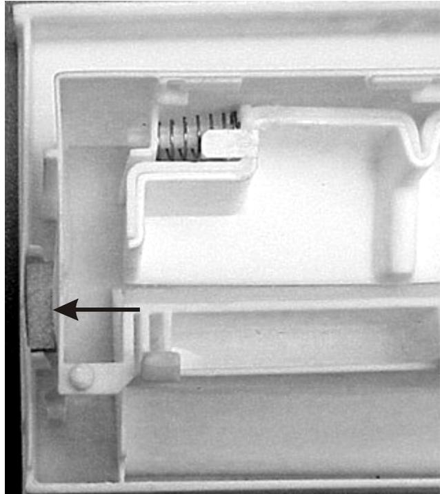
When the drawer is closed, the magnet causes the contacts of the reed switch to close, completing a circuit in the control board.
