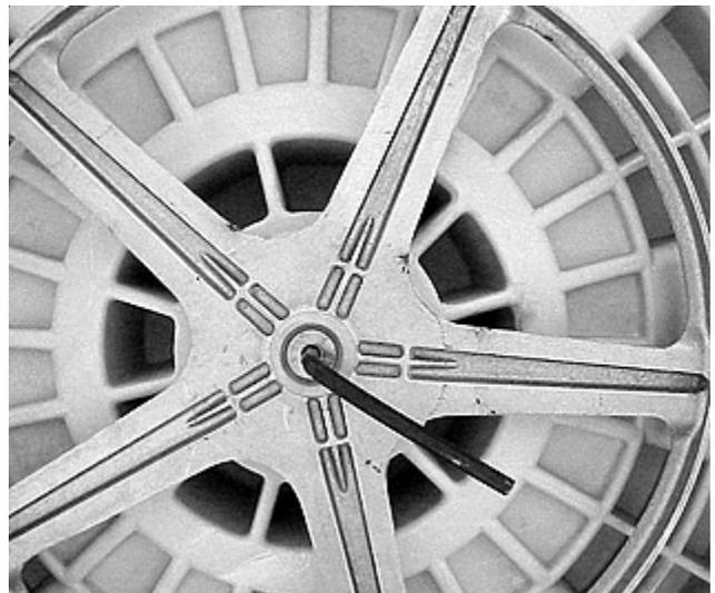
4. Work the pulley back and forth to remove it from the shaft.
