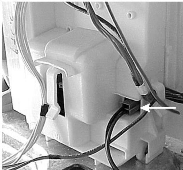
3. Disconnect the wire harness and release the spring loaded locking tab on the side of the control board house. Lift the side of the housing up, slide the assembly to the rear to disengage the front tab and lift the assembly away from the washer base.
