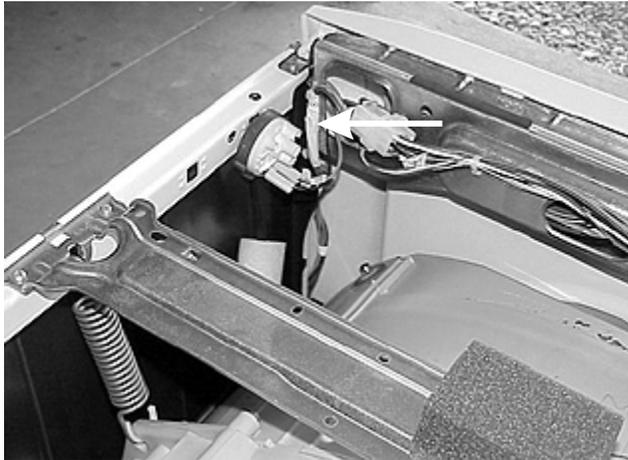
3. Does not have a water temperature sensor.
