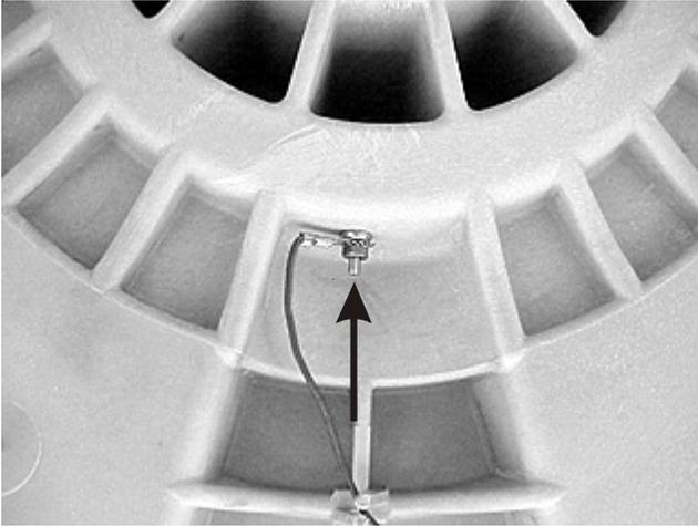
9. Remove the top pins from shock absorbers and push the shock absorbers against the cabinet.
