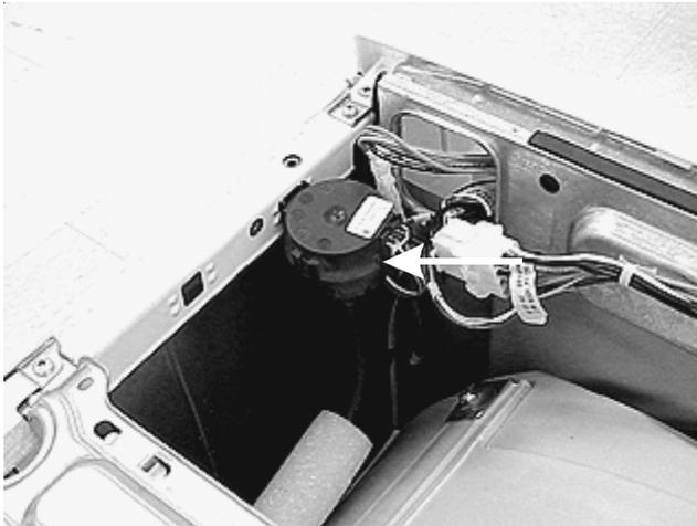
The electronic water level sensor is made up of an electronic board and a bellow inside a sealed chamber. The chamber is connected by a hose to the air bell attached to the drain boot located at the bottom of the washer. The electronic board reads the pressure in the bellow and converts it to an electronic signal. This signal is sent to the control board. The control board controls the incoming water by connecting or disconnecting neutral to the water solenoids.
