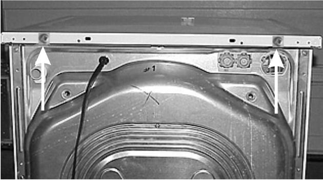
**Removing the pressure switch: (Good Models)**
