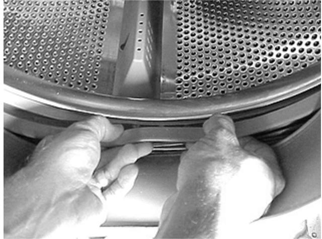
5. Using your thumb, start on the other side of the top tab and force the bellows on in the other direction. Again about one third of the way around stop and seat the bellows onto the tub lip. Then force the remaining bellows on with your thumb and seat it.
