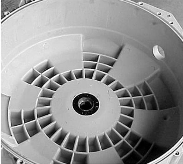
Each vane is locked in place by (4) tabs press out of the spin basket.
