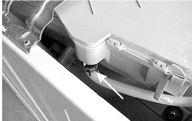
7. Release the (2) tabs, one on each side, locking the housing to the console mounting panel.
