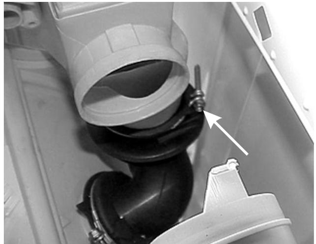
5. Remove the (2) screws holding the housing to the center bar.
