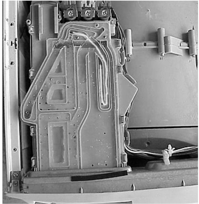
As the water pass over the bleach section, holes in the cavity allows some of the water to enter and mix with the bleach.
