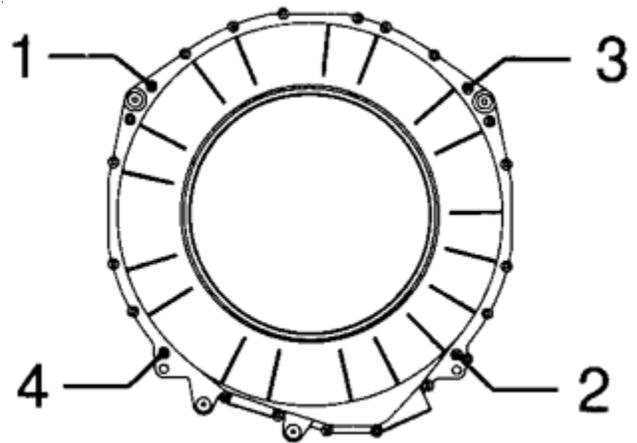
15. The seal between the (2) tub halves is placed in the groove of the rear half and can be lifted out.
