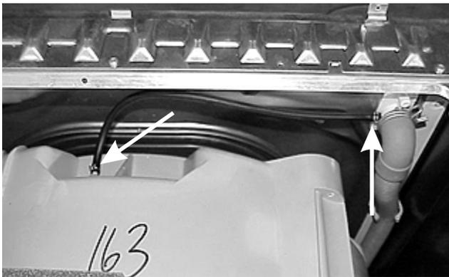
4. Slide the hose off the tub and pump to remove the sump.
