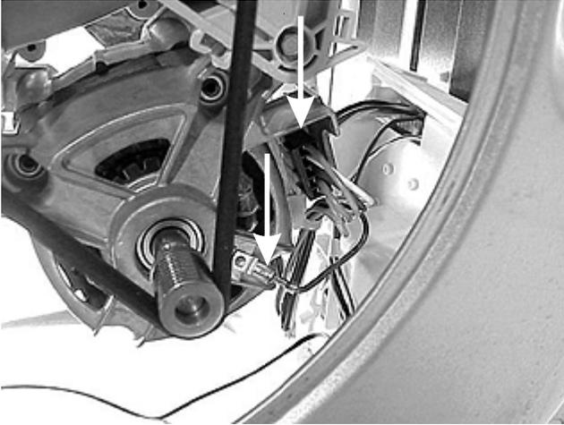
3. Using a 5/16" socket remove the (4) bolts, two in the front and two in the rear, that hold the motor to the outer tub.
