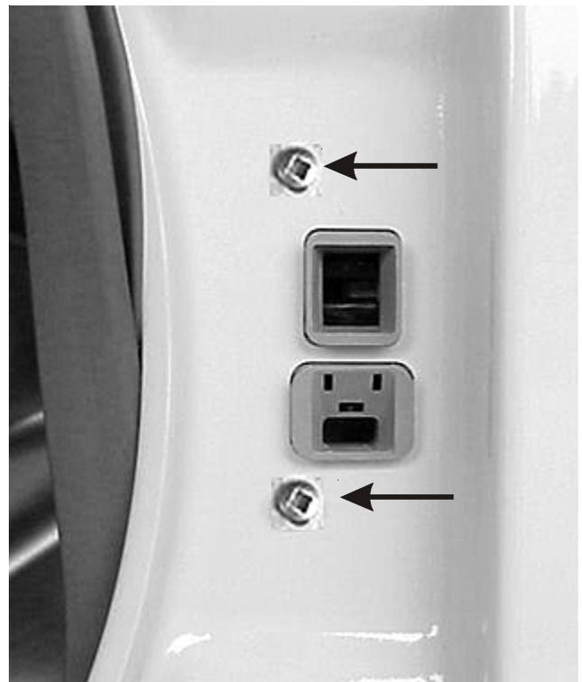
4. Pull the switch assembly into the door opening and unplug the electrical connectors.
