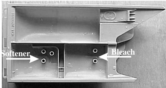
These tubes allow bleach or softener to be added to their cavity without being dispensed as long as the liquid is below the top of the tubes. At the proper time in the cycle when bleach or fabric softener is to be dispensed, water is added to the cavity. This raises the mixture above the top of the tube and the bleach or fabric softener starts flow into the tub.
