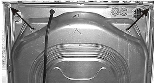
4. Pull back to disengage the (2) tabs and lift the brace off.
