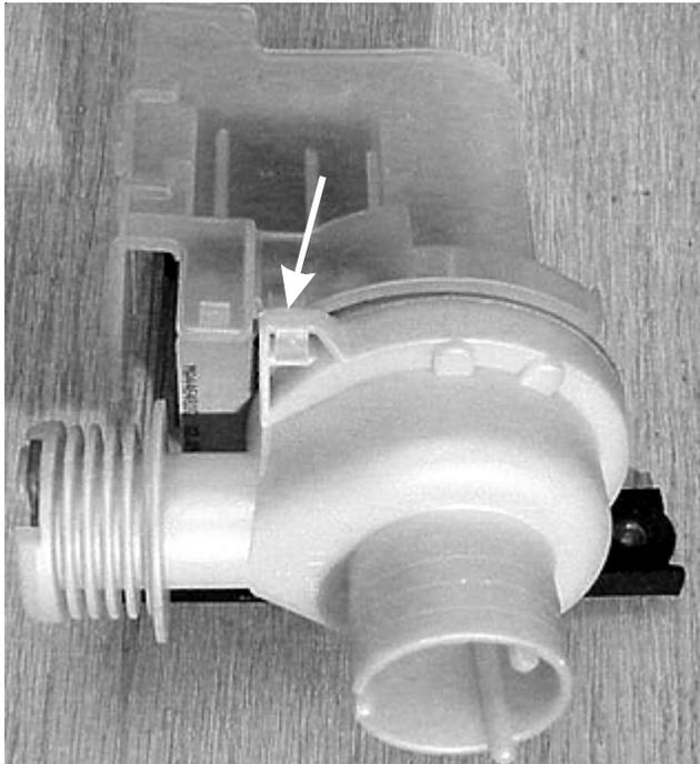
3. Release the tab on each side of the motor and pull back to remove the armature.
