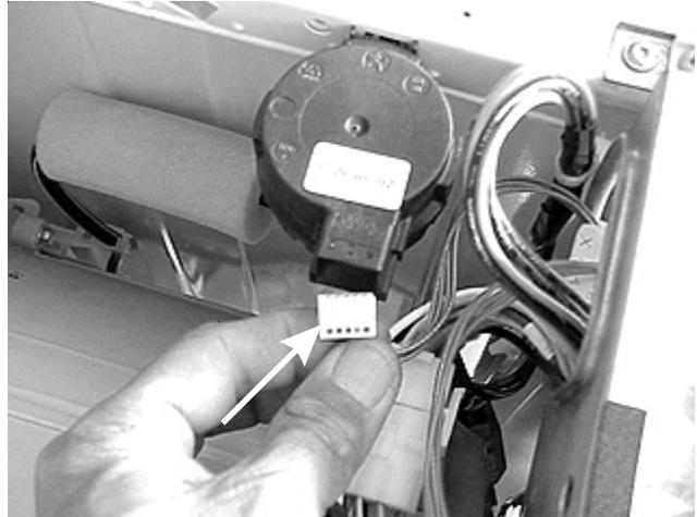
3. Turn the sensor one quarter turn and pull out to release it from the side panel.
