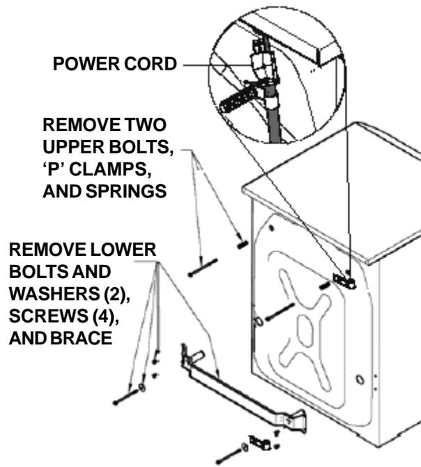
6. Remove the following from the back panel of the washer:
