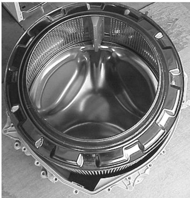
14. Reverse procedure to reassemble using illustration below to show outer tub screw tightening sequence.
