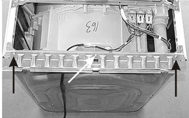
3. Remove the (2) screws from the rear of the brace.
