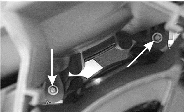
4. Slide motor forward while supporting to remove.
