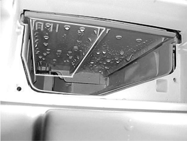
Water in this channel and the mixture from the detergent drawer flow into the tub through the large hose at the rear of the dispenser.
