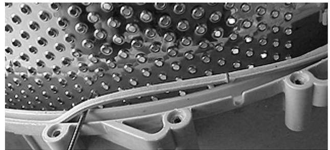
16. To remove the spin basket, set the back half of the outer tub on it's side, and reinstall the screw that secured the large pulley to the shaft. Tap the inner tub out with a rubber hammer.
