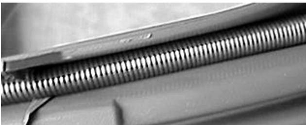
4. Remove the bellows by placing your hand under the bellows at the top of the opening and lift up while pulling out.
