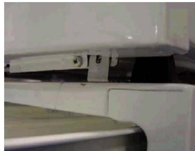
5. Set the dryer down onto the pedestal making sure the service panel bracket on the dryer is behind the front brackets of the pedestal.
