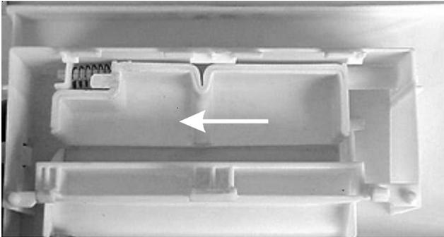
6. To remove the magnet, push the tab to the right with a small screw driver.
