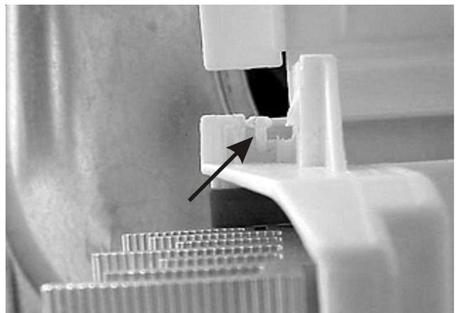
8. Lift the control board out.
