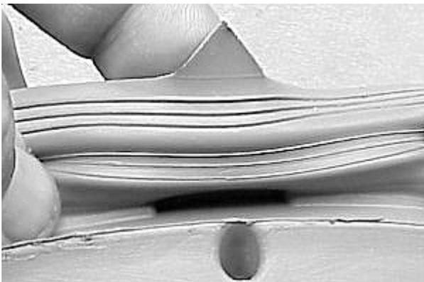
3. Place the slot over the tab and while holding the bellows in place with one hand, place the other hand inside the bellows and force the groove of the bellows over the lip of the tub with your thumb.
