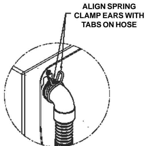
**ORIENT HOSE TO RIGHT, LEFT, UP OR DOWN AS NEEDED BEFORE PLACING CLAMP IN POSITION**
