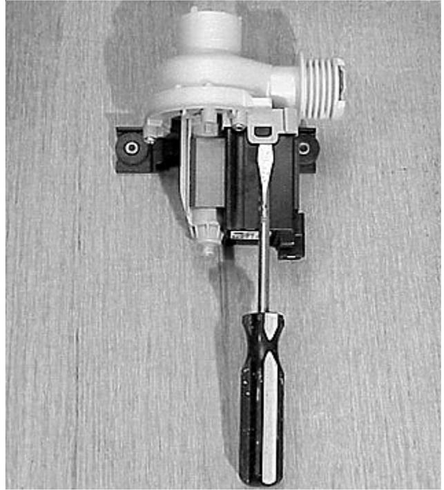
4. Remove (4) screws to release the pump from the housing.
