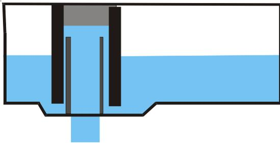
The bleach dispenser channel receives water from the left-hand input, as viewed from the front of the washer. The bleach channel forms a path that allows the water to pass over the bleach section of the cavity
