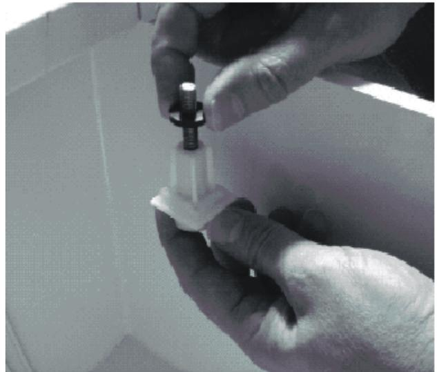
6. Insert the bolt/spacer assembly up through the pedestal with the front spacer positioned in the square hole of the pedestal and the bolt coming through the slotted hole in the washing machine base.
