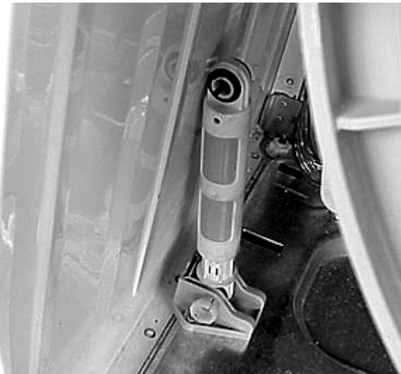
10. Place something down to protect the floor, carefully turn the washer on it's face and release the springs.
