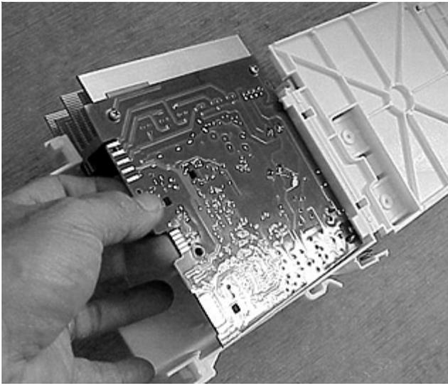
This procedure is much easier if a deep 1/2", 6 point socket (or 13 millimeter, 6 point) is used to compress the locking tab of the plastic pin. Push the socket onto the tapered end of the pin as far as it will go to compress the locking tab.
