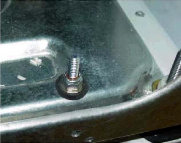
8. Repeat installation of bolt/spacer assembly for the other side.
