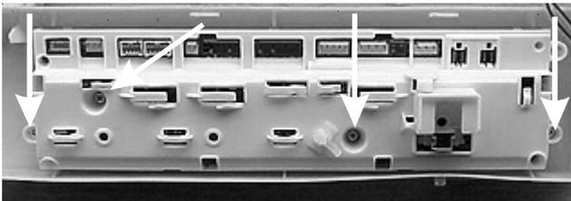
3. Release the locking tabs and lift the control from the console.
