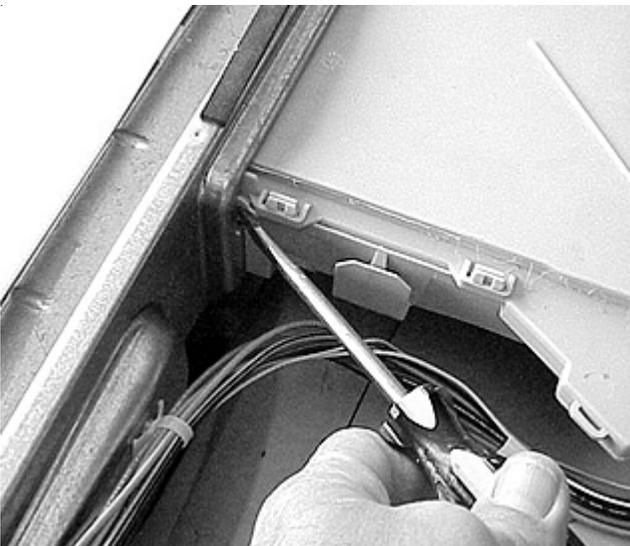
10. Push down on the tub and swing the front of the housing toward the center of the washer. Work the housing out from under the center brace and lift the housing out.
