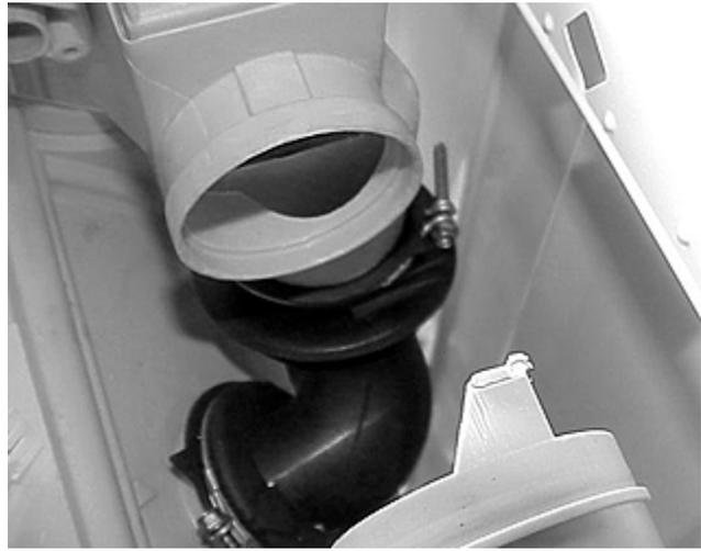
Since the flow of the incoming water is more than the holes can dispense, the excess water backs up into a channel across the rear of the dispenser.
