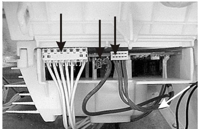
7. To remove the control board from the housing, release the latch on each end at the top and lift the back open.
