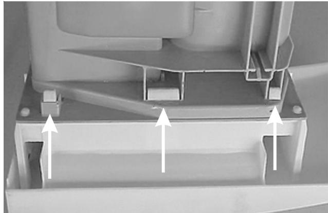
4. To remove the conveyor release the conveyor from the tabs and lift it off.
