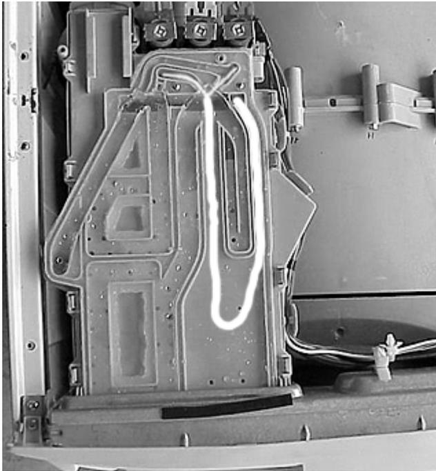
As the water passes over the fabric softener section, holes in the cavity allows some of the water to enter and mix with the fabric softener.
