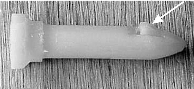
4. Use pliers to grasp head of pin and pull to remove. As the pin is removed, the socket will drop free.
