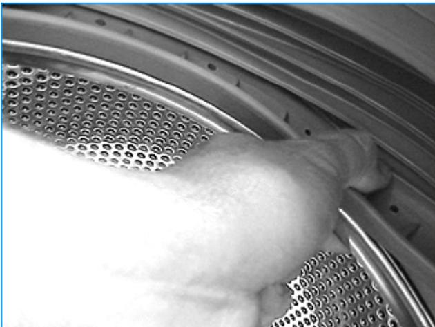
4. Work your way about one third way around the tub, then pull in on the inside flap of the bellows to seat the bellows into the lip of the tub.
