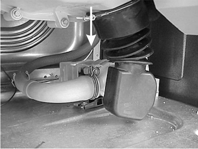
3. Release the and slide the hose off the drain hose coupler.
