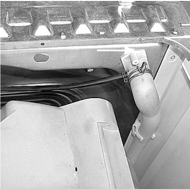
5. Release the hose from it guides and pull the hose out.
