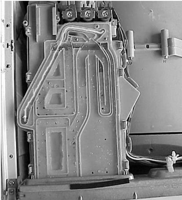
This path allows the water to bypass the dispenser drawer and enter the tub by an advanced rinsing technology hose connected between the cavity and the bellows.
