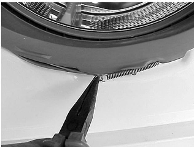
3. Pull the bellows off of the lip of the front panel.
