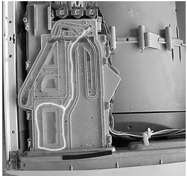
As the water pass over the detergent section, holes in the cavity allows some of the water to enter and flush the detergent cavity.
