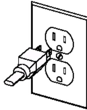
**NOTE:** GFI (Ground Fault Interrupter) receptacle is not required.
