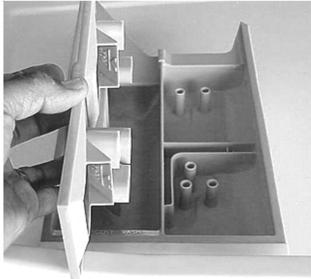
3. To remove the drawer front, release the three tabs and pull the drawer front away from the body. When replacing the drawer front always remember to transfer the reed switch magnet.
