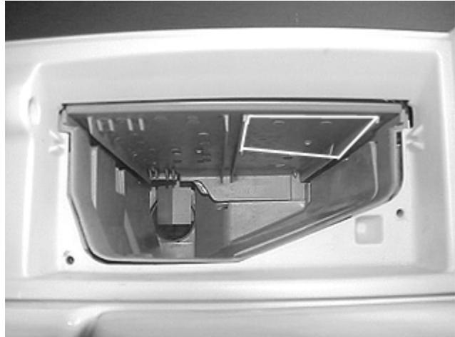
This raises the mixture level above the tubes in the drawer fabric softener cavity allowing the mixture to flow into the tub. Like the detergent channel, the flow of the incoming water is more than the holes can dispense. The excess water backs up into the channel across the rear of the dispenser and flows into the tub.
