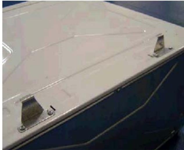
3. Attach the front brackets to the pedestal with four #8 screws (2 per bracket).
