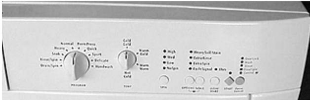
2. Water fill height control is a pressure switch.
