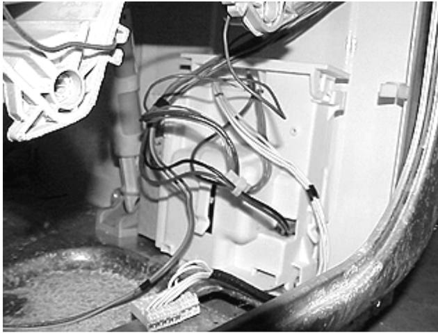
**Note:** The control board is mounted in the console. The speed control board is mounted in the left rear corner of the washer.
