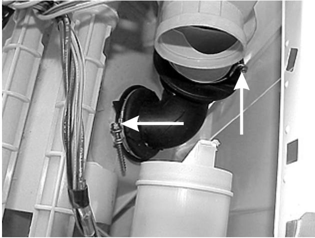
2. Loosen the clamp at the tub.
