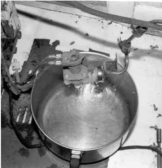
Fig. 09-07 Testing a Icemaker Valve with a Homemade Line Cord
