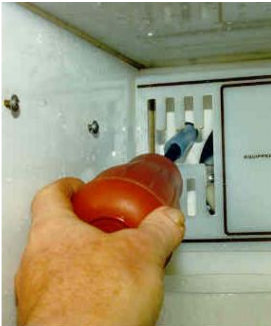
Fig. 09-06 Thawing a Frozen Spout
