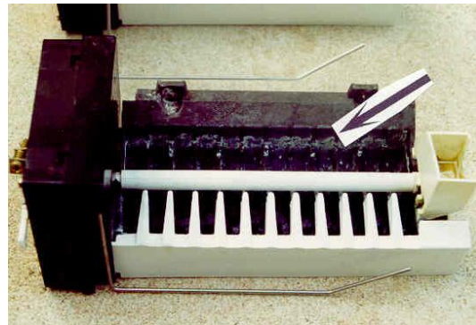
Fig. 092_15 Corrosion on a Mold
