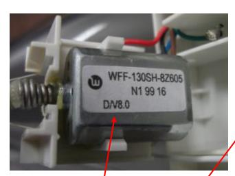
Door locked by. Reed Switch in blue plastic **Door Lock Replaced as an Assembly.**
