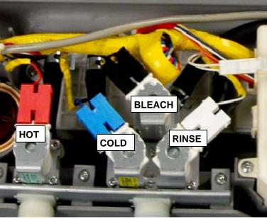
Softener is dispensed in the final rinse by the "RINSE" valve. This valve is only used to dispense the Sof-
