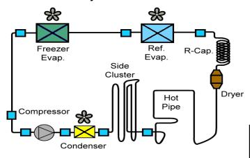
Compressor  $\rightarrow$  Condenser  $\rightarrow$  Side Cluster  $\rightarrow$  Hot Pipe  $\rightarrow$  Dryer  $\rightarrow$  R Capillary  $\rightarrow$  R Evaporator  $\rightarrow$  F Evaporator  $\rightarrow$  Suction Pipe  $\rightarrow$  Compressor
