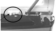
The **Door Switch** must always be on the side the hinge is on. If not, the Fridge door may not always close properly, creating an intermittent Fridge no or poor cooling.
