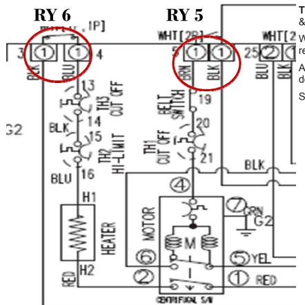
**Testing Main PCB power** output to Heating & Motor circuit.
