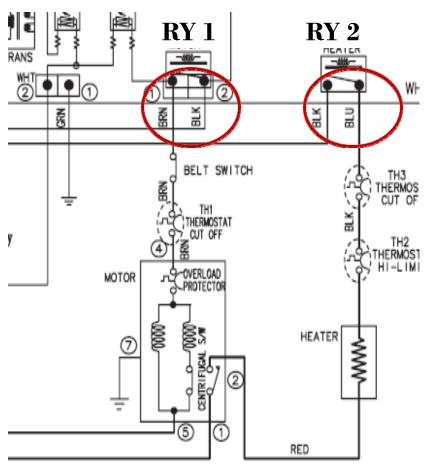
**Testing Main PCB power** output to Heating & Motor circuit.
