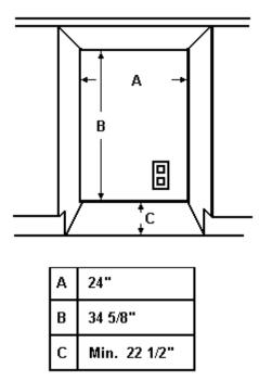
24" width for cabinet only. 24 1/4" needed for cabinet and door width clearance if door is to be recessed between cabinets.
