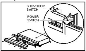
After power is initially plugged in, after a power loss, or if power switch is turned off, all temperature indicator lights will flash until Alarm Off or Display On is pressed.
