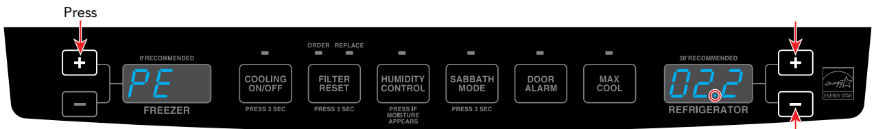
Press either button to scroll through the numbers until the proper number is in the display
