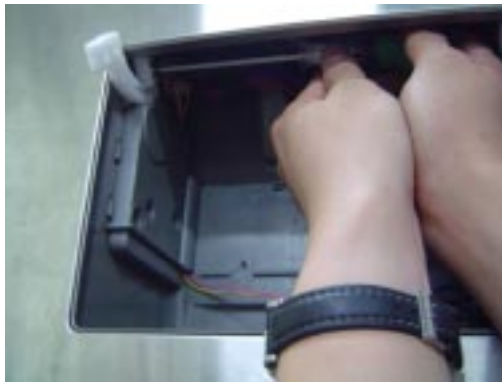
16) Unscrew the 1 screw at the gear ( left and right)
