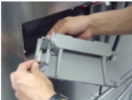
12) Separate the Switch connection harness.
