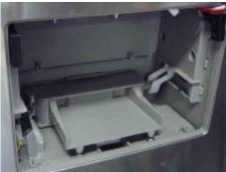
11) Before separation of Bracket, connecting rod have to be at back side position.
