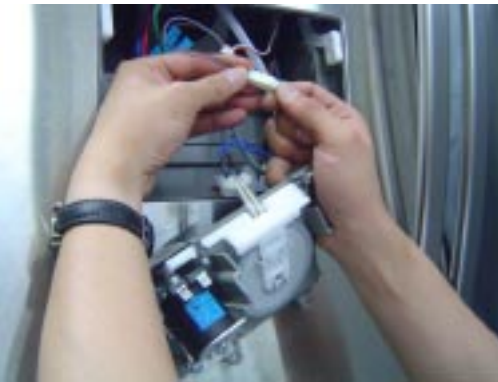
15) All harness have to be separated.
