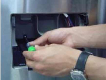
7) Unscrew 2 points to separate tray-cover
