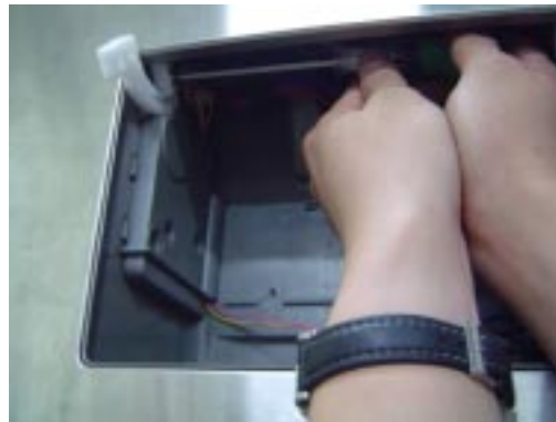
16) Unscrew the 1 screw at the gear ( left and right)
