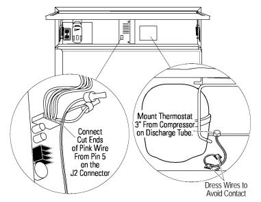
**Note:** Allow approximately 20 minutes for the condenser fan to turn on after the compressor starts.
