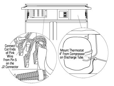
**Note:** Allow approximately 20 minutes for the condenser fan to turn on after the compressor starts.
