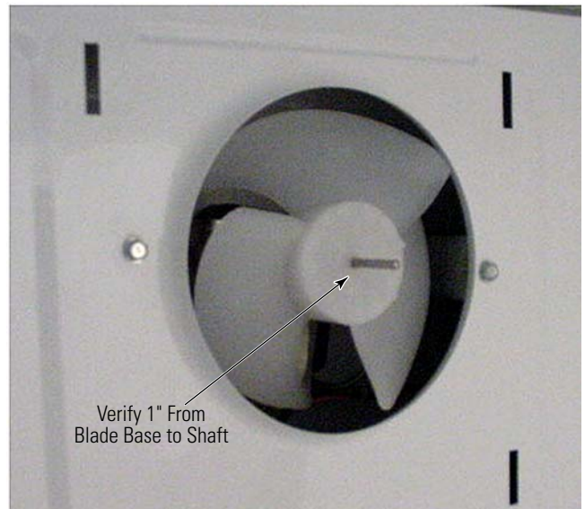
Figure 2 Verify measurement of 1" from blade base to shaft
