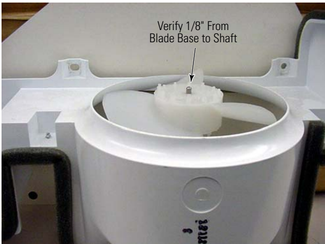
Figure 1 Verify measurement of 1/8" from blade base to shaft
