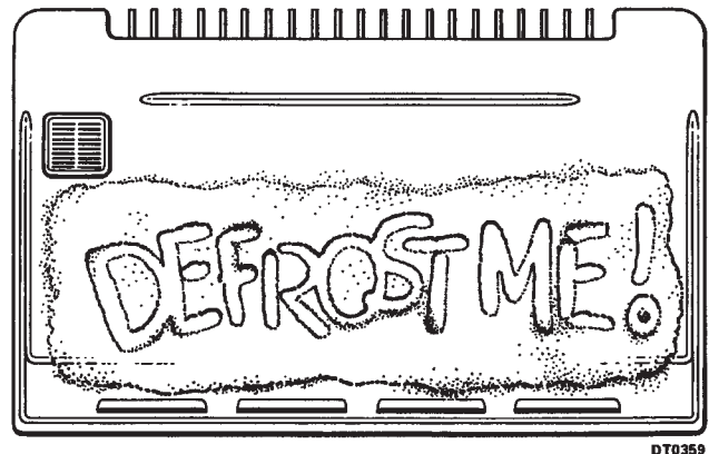
Figure 5 - Excessively Frosted Evaporator
