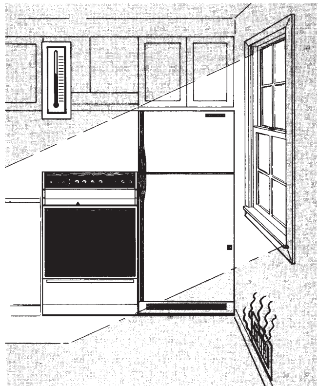
Figure 9 - Improper Installation Location
