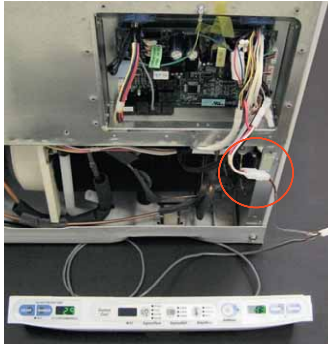
Diagnostic Aid - Main Board Access
