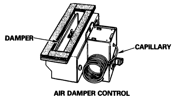
Figure 27 - Automatic Air Control
