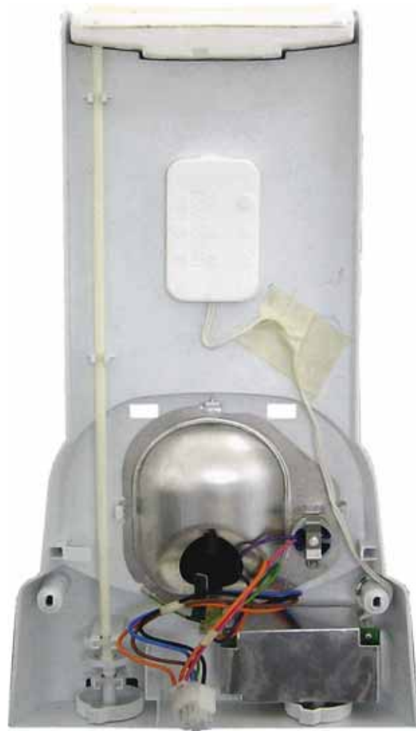
Control Housing Removed
