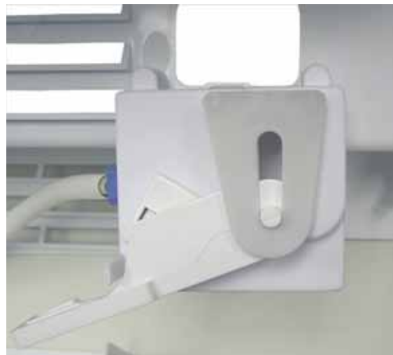
BIN FULL - SWITCH OPEN POSITION
