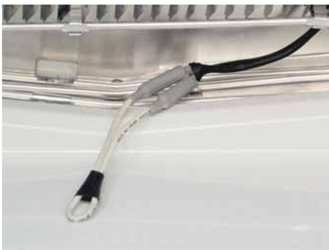
Drain heater removed from drain
