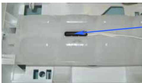
Icemaker sensor located under insulated pad.
