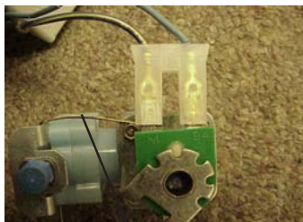
Terminal on Coil is Installed
