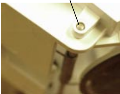
Use a small punch to remove shaft.
