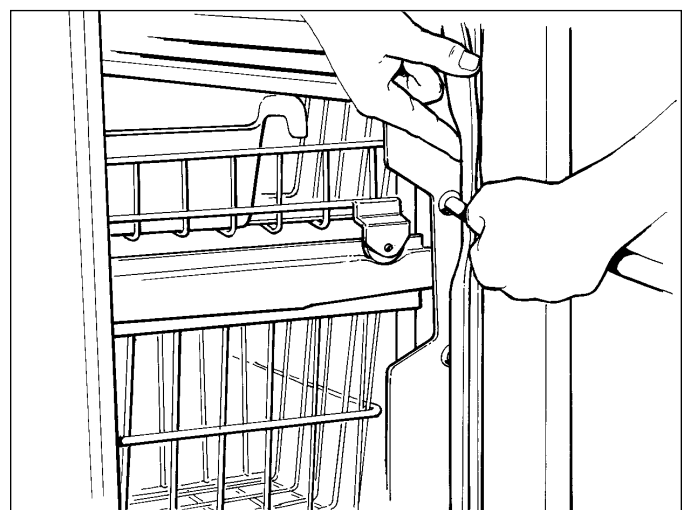
Figure 2-10. Drawer Front Pitch Adjustment
