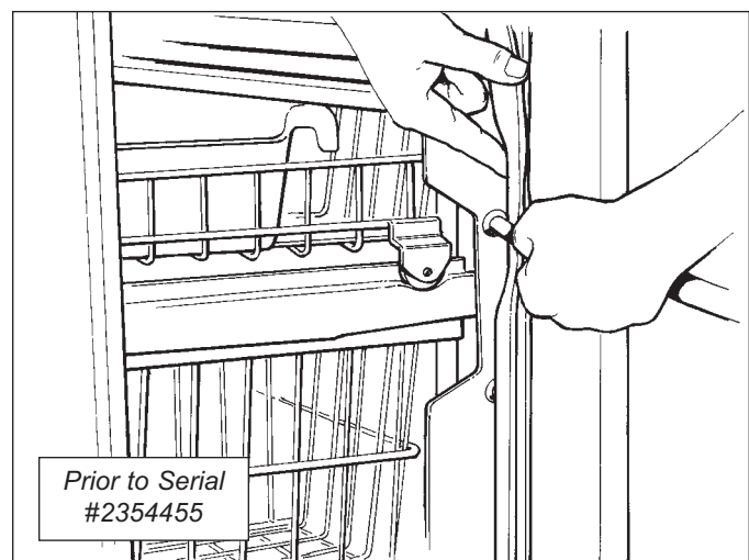
Figure 2-10. Drawer Front Pitch Adjustment
