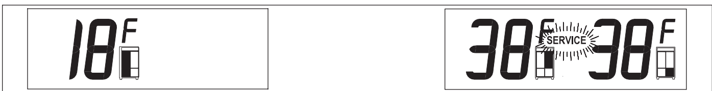
Figure 3-27. SERVICE Flashing = Several Excessive Compressor Run Periods
