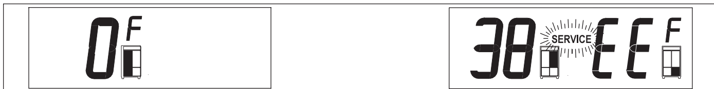
Fig. 3-36. “EE” at Right of Right User Display & “SERVICE” Flashing = Lower Ref. Zone Thermistor Fault
