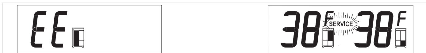
Figure 3-34. “EE” in Left User Display, SERVICE Flashing in Right = Freezer Zone Thermistor Fault
