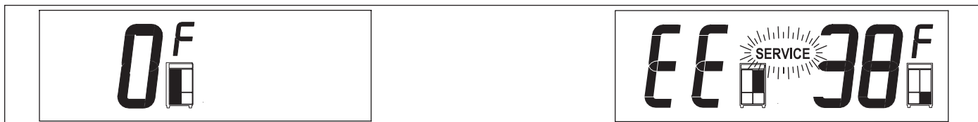
Figure 3-35. “EE” at Left of Right User Display & “SERVICE” Flashing = Upper Ref. Zone Thermistor Fault
