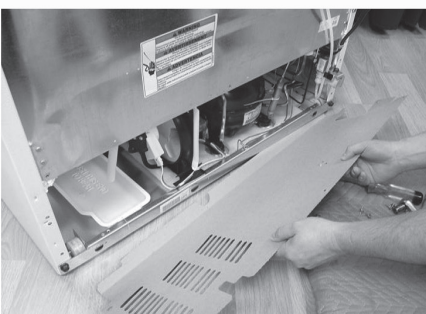
5. Remove machine compartment screws and remove cover
