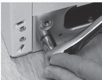
3. Remove 1/2" bolts on left and right hand sides Remove grille
