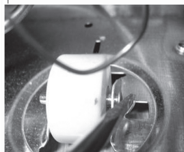
1. Fold the locking tab down to allow the axle to be removed from the roller and bracket.
