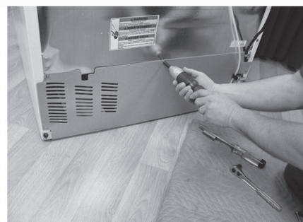
5. Remove machine compartment screws and remove cover
