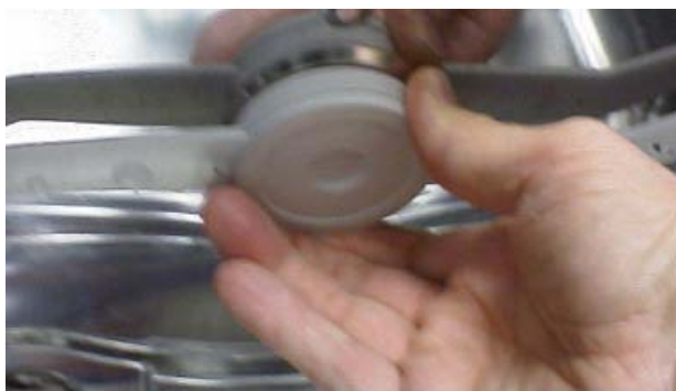
Turn center of spray arm to remove
